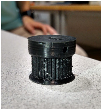
3D printed pulley with support artifacts remaining
